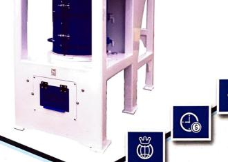
Perfect's modified whitener is specially designed for effective degree of whiteness and maximum yield of head rice with less percentage of broken rice. The rice is whitened very gently between abrasive grinding wheel & screen without distracting the original shape of rice kernel. This machine is equipped with a mechanism for adjusting degree of whiteness.
