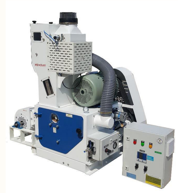
SPV – Vibro Pneumatic Sheller (3 – 6 TPH)
